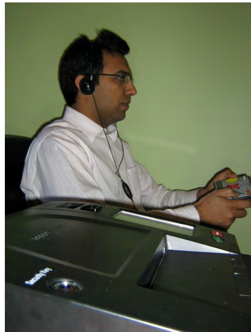
Ballot Marker Device for Accessible Voting – Marks a Paper Ballot
