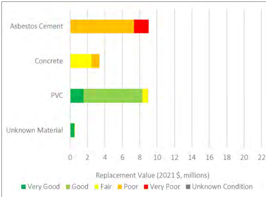
Figure 4-38: Condition by Replacement Value – Arthur Wastewater Mains
